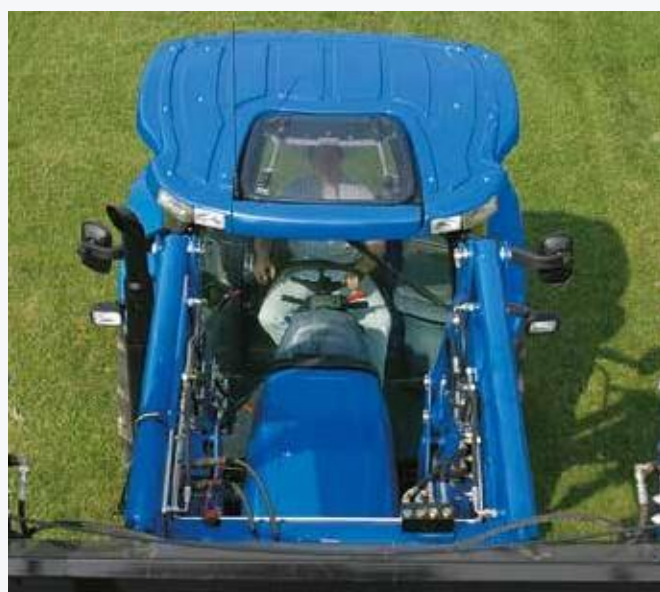
The Horizon™ cab features an optional high-visibility roof panel for an easy view to a raised loader bucket.
