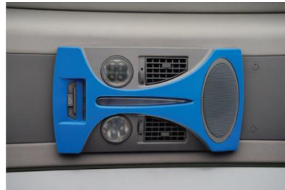
Reading lights, individual A.C. controls
